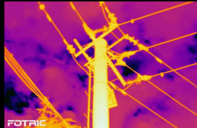
640*480 IR resolution (25° lens at 30m distance)
